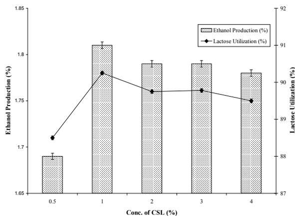
**Figure 2:** Effect of corn steep liquor concentration on ethanol production and lactose utilization from whey using *K. marxianus* WIG 2
