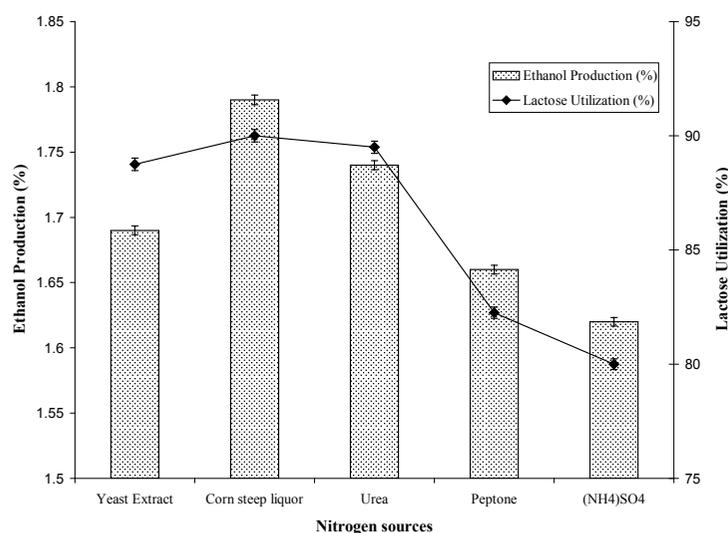
**Figure 1: Screening of nitrogen sources for ethanol production and lactose utilization from whey using *K. marxianus* WIG 2**
