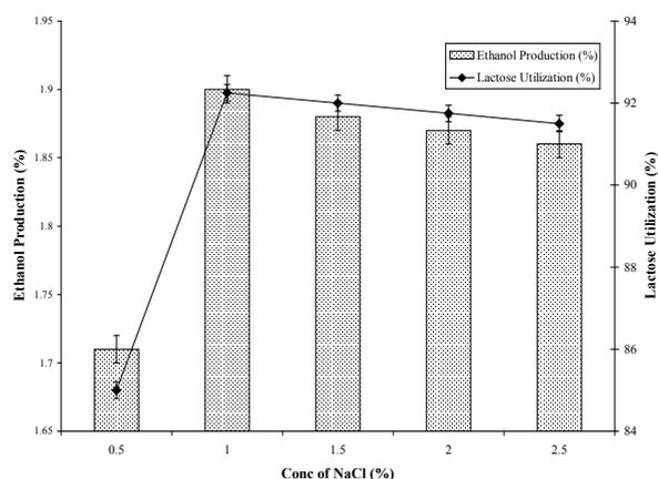
**Figure 4:** Effect of  $\text{NaCl}$  concentration on ethanol production and lactose utilization from whey using *K. marxianus* WIG 2
