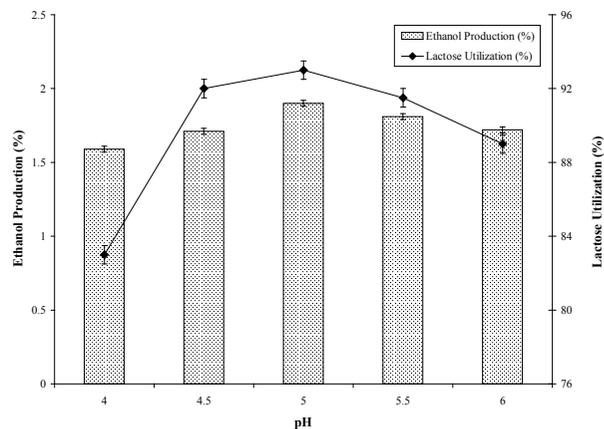
**Figure 5:** Effect of pH on ethanol production and lactose utilization from whey using *K. marxianus* WIG 2
