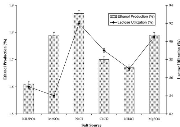
**Fig 3:** Effect of different salts on ethanol production and lactose utilization from whey using *K. marxianus* WIG 2
