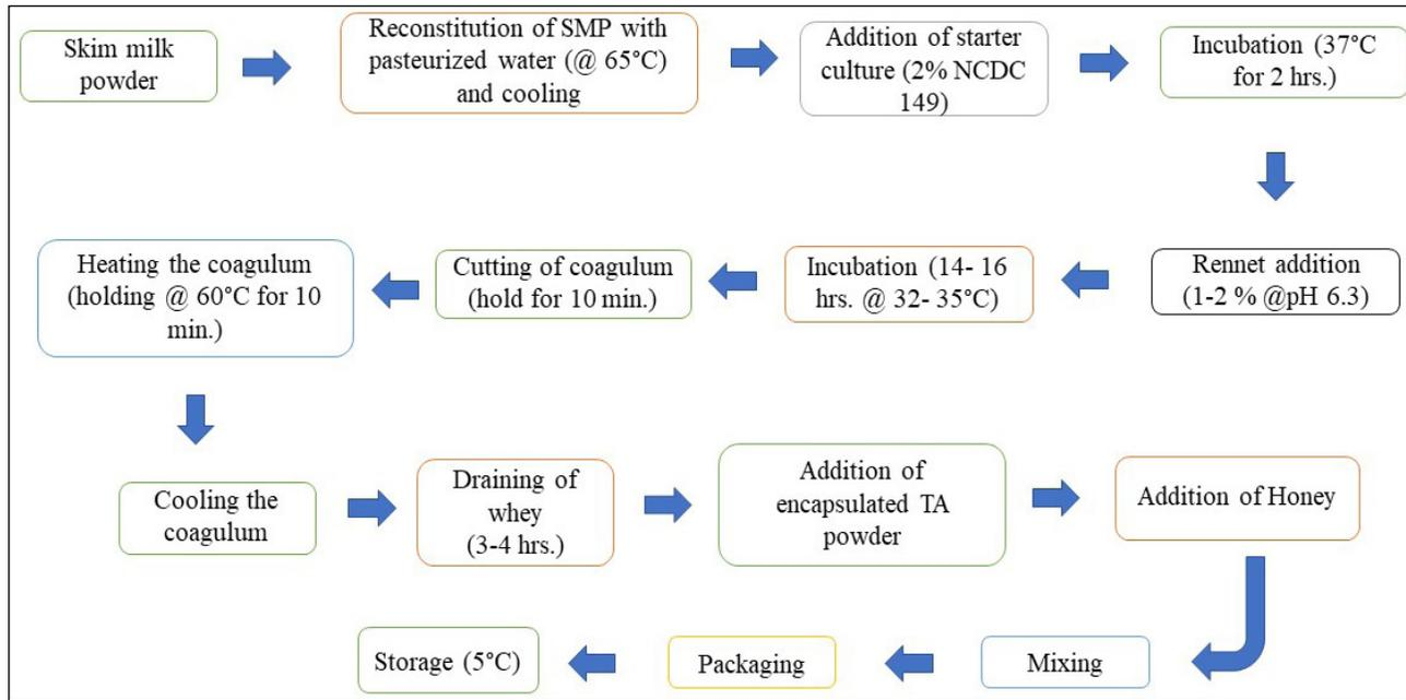
**Fig. 1:** Process diagram for encapsulated Arjuna incorporated Quarg-type cheese
