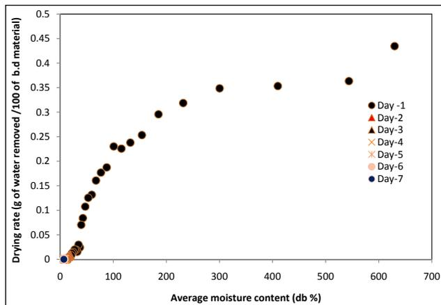
**Fig. 2:** Drying rate (g water removed/100 g of bone dry material/min) versus moisture content % (db) of beetroot slices dried by open sun drying
