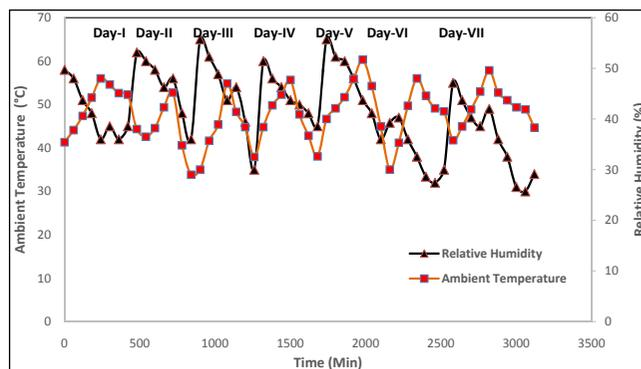
**Fig. 4:** Variation in ambient temperature and relative humidity with time in open air sun drying of beetroot slices
