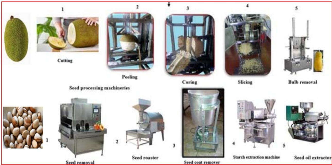
Fig. 5: Machineries used for Jackfruit and Seed Processing
