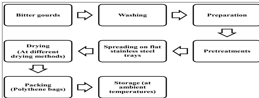
Fig. 1: Flow Chart for Drying of Bitter gourd
