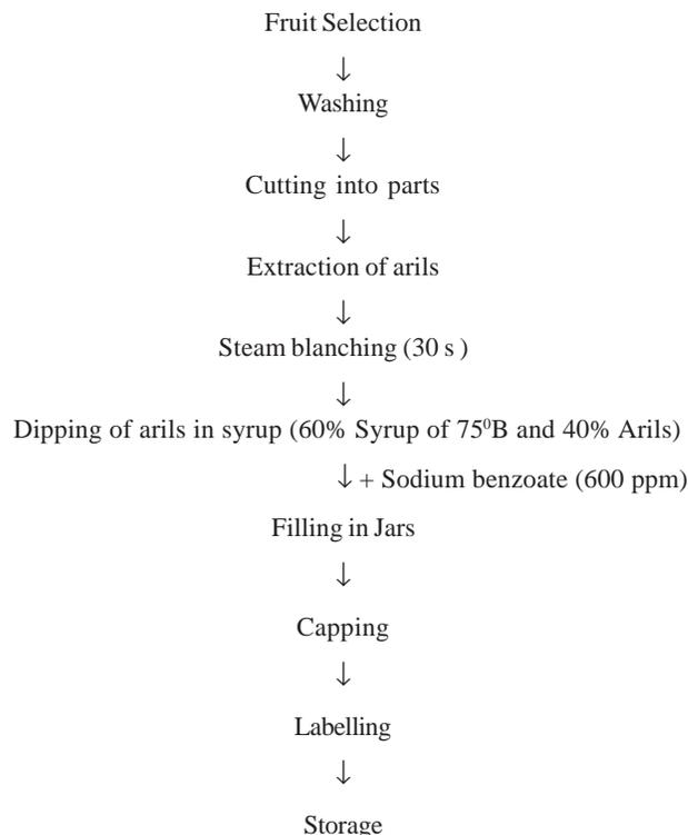
**Fig. 1:** Unit operations for the preparation of arils in syrup from wild pomegranate
