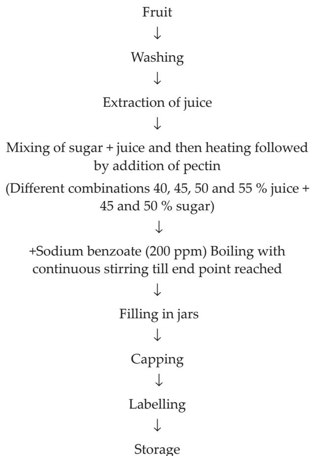
**Fig. 1: Unit operations for the preparation of mulberry jelly**
