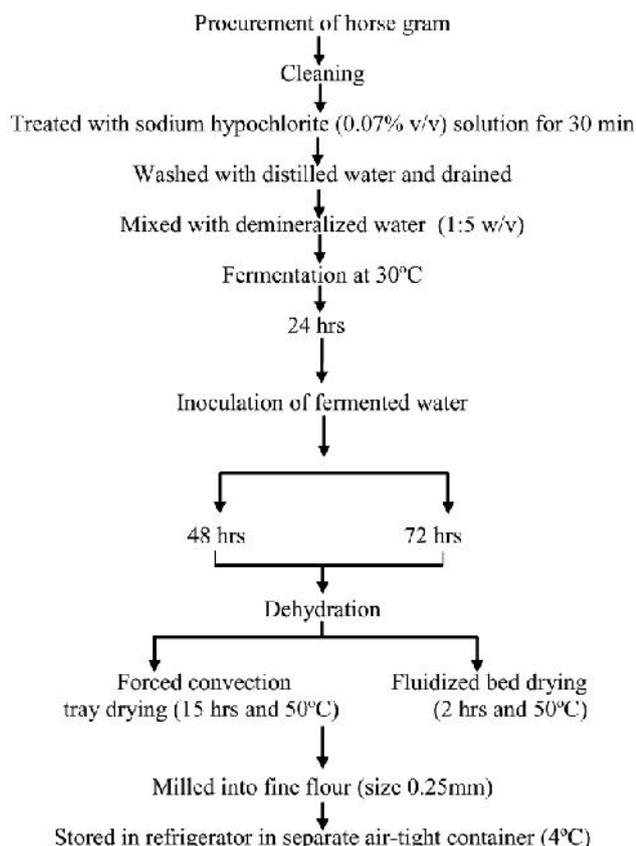
Fig. 1: Flow diagram of process for fermentation and dehydration of horse gram
