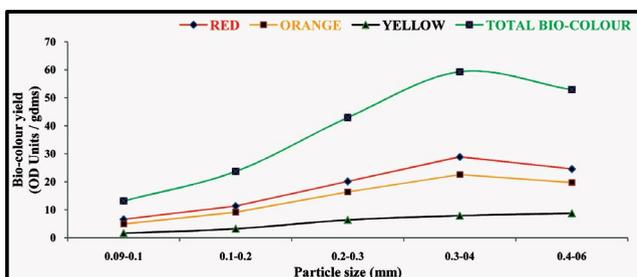
Fig. 3: Effect of particle size on bio-colour yield at 30°C with 2% inoculums (7 days old) pH 6 with 12 days of incubation and 70% (w/v) moisture content
