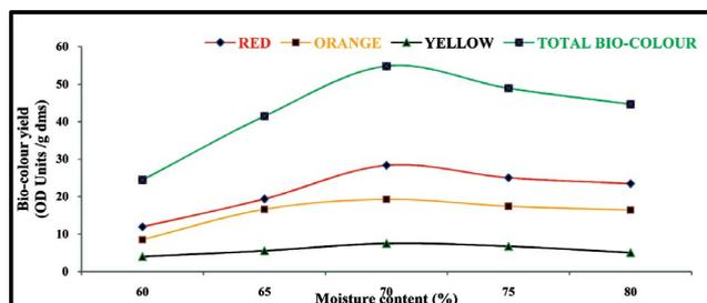
Fig. 2: Effect of moisture content on bio-colour yield at 30°C with 2% inoculums of 7 days old of pH 6 for 12 days of incubation
