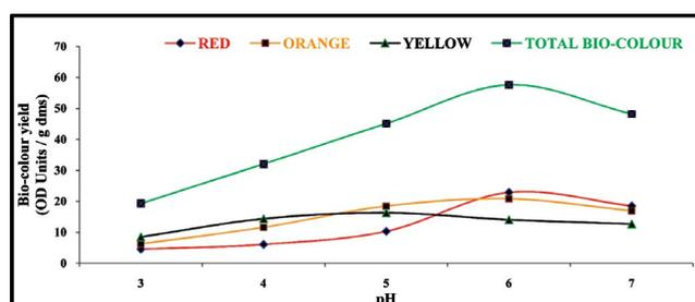
**Fig. 8:** Effect of pH on bio-colour yield at 70% (w/v) moisture content, 0.3-0.4 mm particle size, 30°C with 3% spore suspension of 6 days old inoculums for 9 days of incubation
