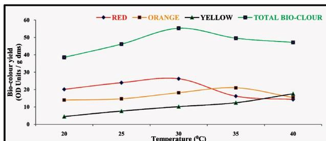
Fig. 4: Effect of temperature on bio-colour yield at 70% (w/v) moisture content, 0.3-0.4 mm particle size with 2% inoculums of 7 days old of pH 6 for 12 days of incubation
