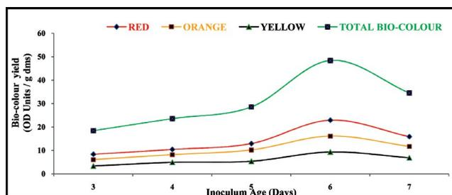
Fig. 5: Effect of inoculums age on bio-colour yield at 70% (w/v) moisture content, 0.3-0.4 mm particle size, 30°C with 2% inoculum of pH 6 for 12 days of incubation
