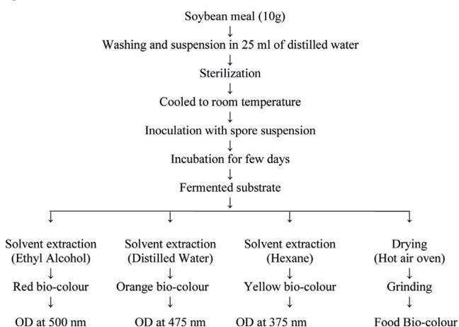
Fig. 1: Production of bio-colour using soybean meal as a substrate through solid state fermentation
