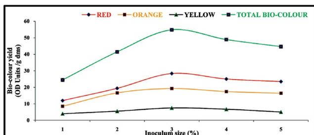
**Fig. 6:** Effect of inoculum size on bio-colour yield at 70% (w/v) moisture content, 0.3-0.4 mm particle size, 30°C with 6 days old inoculums of pH 6 for 12 days of incubation
