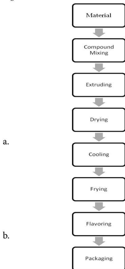
Fig. 1: Process flow chart of making non-veg extruded chips
