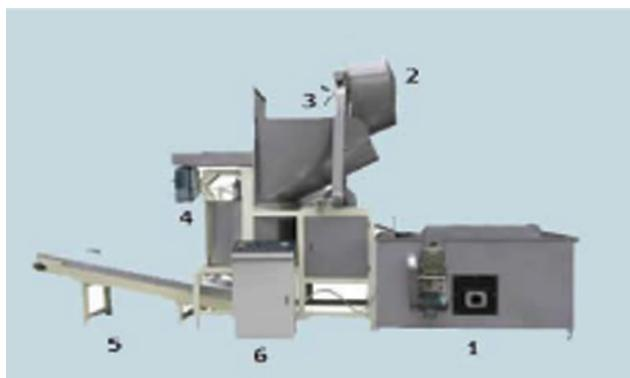
**Fig. 4: Fryer.** In the figuer, 1. Fryer, 2. Material Basket, 3. Rise and Fall Device, 4. Deoiling Machine, 5. Output Conveyor, 6. Controlling Panel
