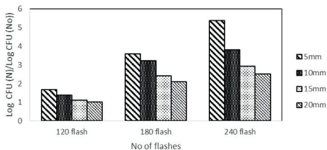
**Fig. 3: Effect of layer depth(mm) on bacterial inactivation at a distance of 5cm from the lamp**
