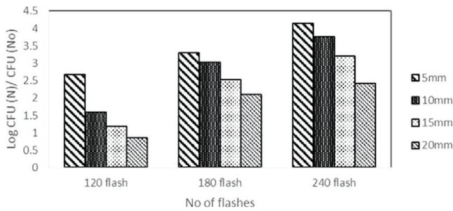
**Fig. 6: Effect of layer depth (mm) on Yeast and mold inactivation at a distance of 5 cm from the lamp**
