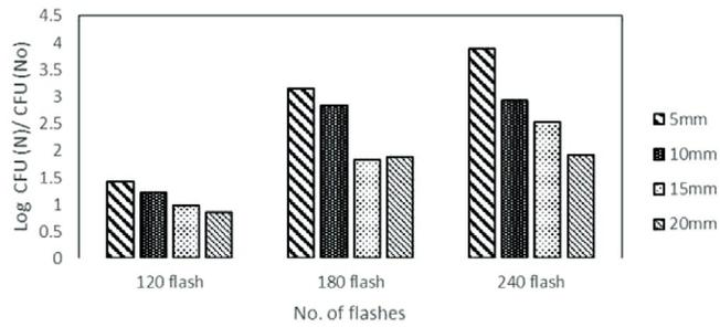
**Fig. 4: Effect of layer depth (mm) on bacterial inactivation at a distance of 10 cm from the lamp**
