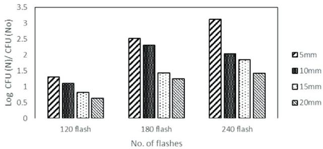
**Fig. 5: Effect of layer depth (mm) on bacterial inactivation at a distance of 15 cm from the lamp**
