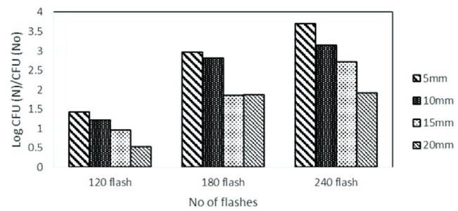
**Fig. 8: Effect of layer depth (mm) on Yeast and mold inactivation at a distance of 15 cm from the lamp**
