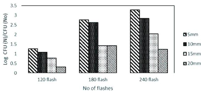
**Fig. 7: Effect of layer depth (mm) on Yeast and mold inactivation at a distance of 10 cm from the lamp**
