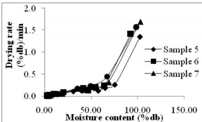
Fig. 3 (b) Variation of drying rate with moisture content for sample 5, 6, 7 and 8.
