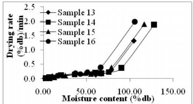
Fig. 3 (d) Variation of drying rate with moisture content for sample 13, 14, 15 and 16.
