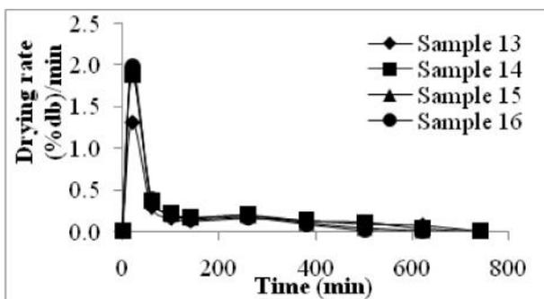
Fig. 2 (d) Variation of drying rate with drying time for sample 13, 14, 15 and 16.
