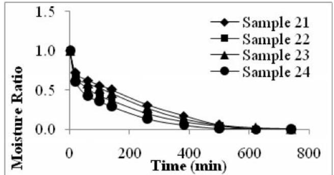
Fig. 1 (f) Variation of Moisture ratio with drying time for sample 21, 22, 23 and 24.
