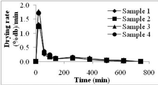
Fig. 2 (a) Variation of drying rate with drying time for sample 1, 2, 3 and 4.
