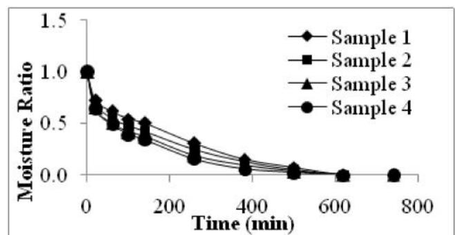
Fig.1(a) Variation of Moisture ratio with drying time for sample 1, 2, 3 and 4.
