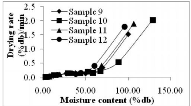
Fig. 3(c) Variation of drying rate with moisture content for sample 9, 10, 11 and 12.
