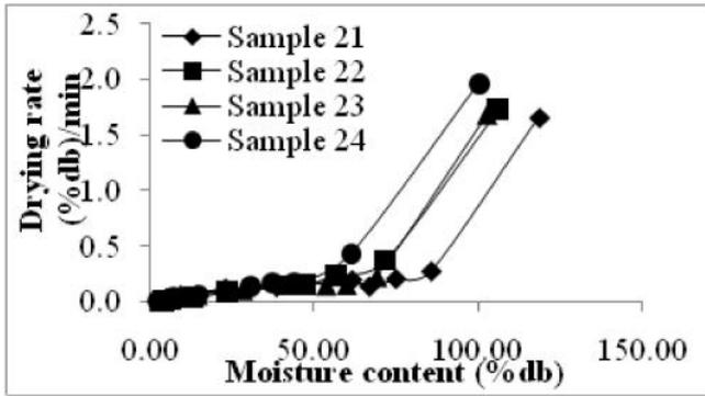
Fig. 3 (f) Variation of drying rate with moisture content for sample 21, 22, 23 and 24.
