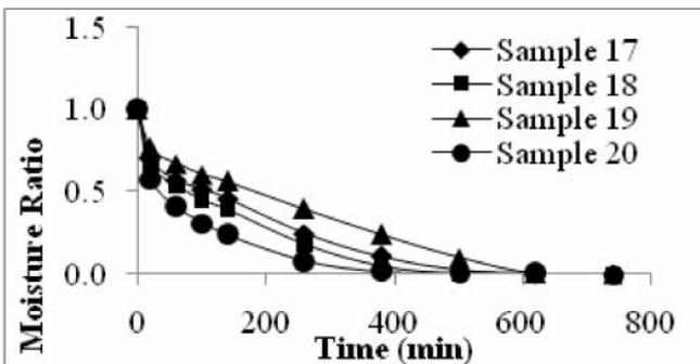
Fig. 1 (e) Variation of Moisture ratio with drying time for sample 17, 18, 19 and 20.
