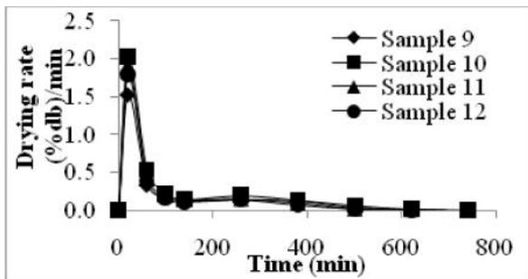
Fig. 2 (c) Variation of drying rate with drying time for sample 9, 10, 11 and 12.
