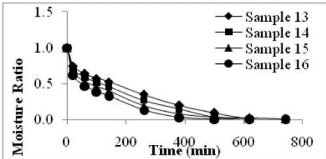
Fig. 1(d) Variation of Moisture ratio with drying time for sample 13, 14, 15 and 16.
