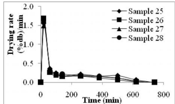
Fig. 2 (g) Variation of drying rate with drying time for sample 25, 26, 27 and 28.
