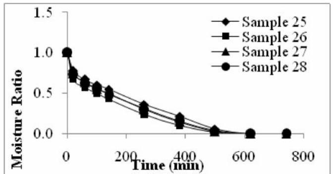
Fig. 1 (g) Variation of Moisture ratio with drying time for sample 25, 26, 27 and 28.
