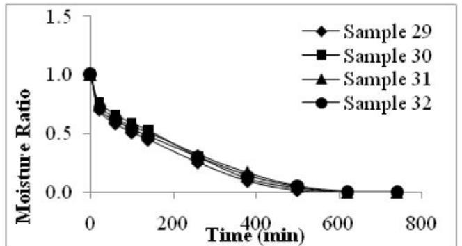
Fig. 1 (h) Variation of Moisture ratio with drying time for sample 29, 30, 31 and 32.
