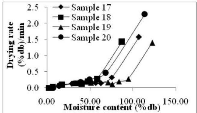
Fig. 3 (e) Variation of drying rate with moisture content for sample 17, 18, 19 and 20.
