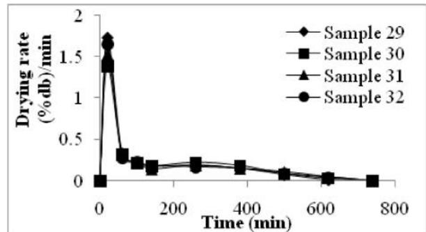
Fig. 2 (h) Variation of drying rate with drying time for sample 29, 30, 31 and 32.
