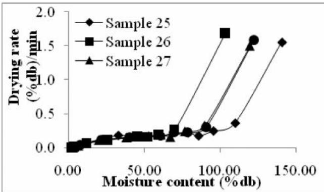
Fig. 3 (g) Variation of drying rate with moisture content for sample 25, 26, 27 and 28.
