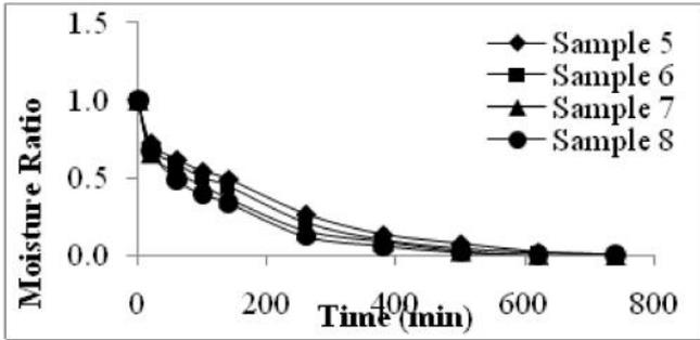
Fig. 1(b) Variation of Moisture ratio with drying time for sample 5, 6, 7 and 8.
