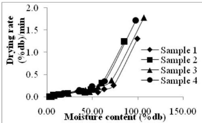
Fig. 3 (a) Variation of drying rate with moisture content for sample 1, 2, 3 and 4.
