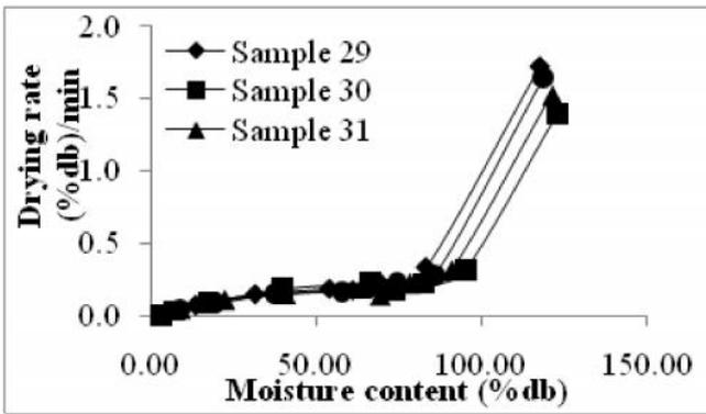
Fig. 3(h) Variation of drying rate with moisture content for sample 29, 30, 31 and 32.
